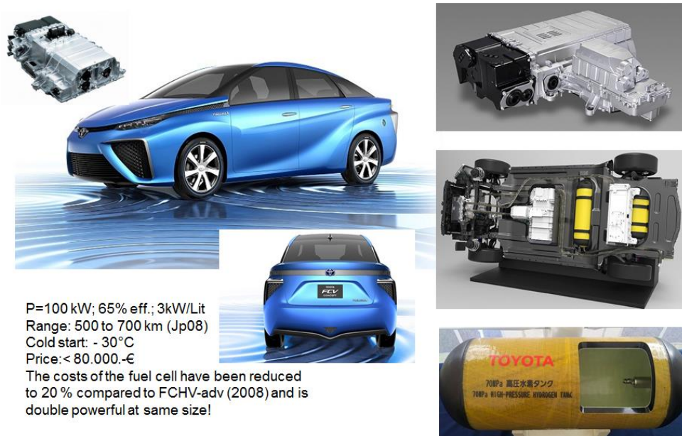
Figure 14: Toyota "MIRAI" (=Future) vehicle and FC components
