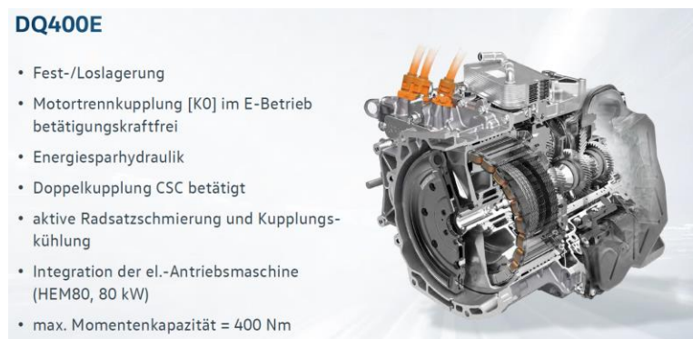
Figure 24: Example VW DQ400E "Hybrid"Transmission
